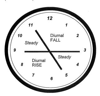
The easiest way to remove diurnal change from your calculations is to read your barometer at the SAME TIME of the day, preferably at about 10 or 4 (am or pm), thus observing pressure change over 24-hour periods. Remember to log the pressure and its
