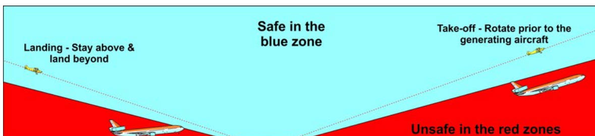
Fig. 86 Safe Zones (blue) for Landing and Take-off in relation to Wake Turbulence Generated by other Aircraft.
