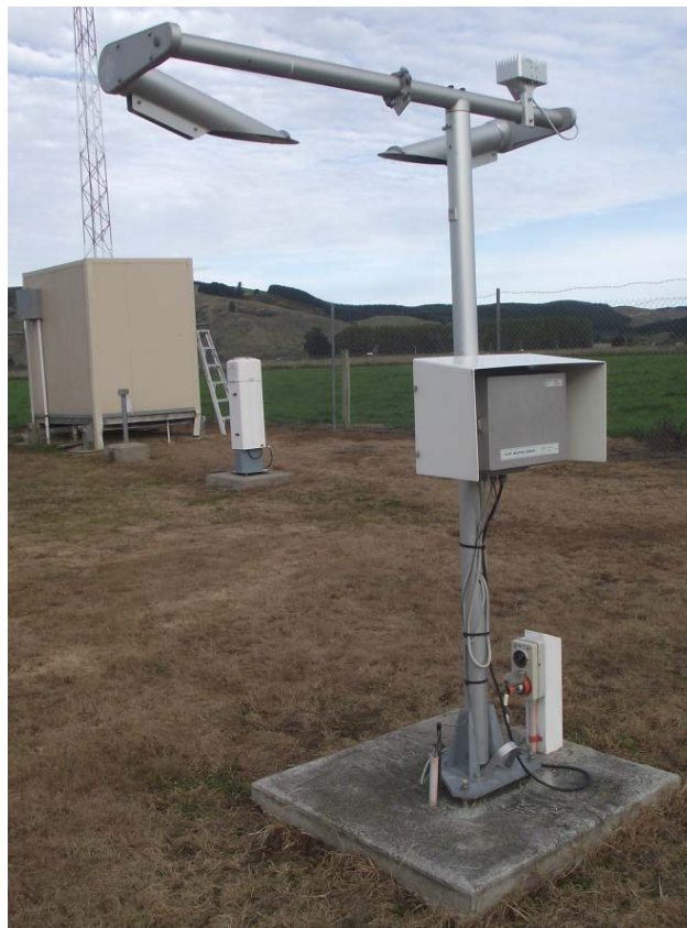
Fig. 69 A Forward Scatter Visibility Meter.
