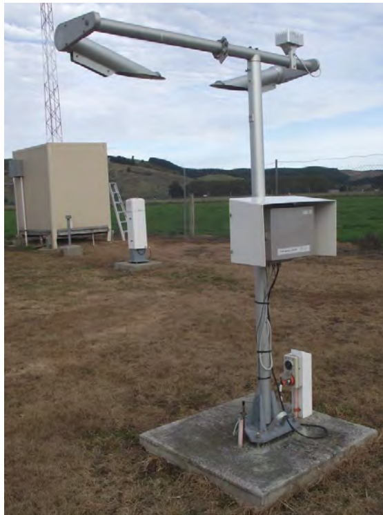
Fig. 69 A forward scatter visibility meter.
