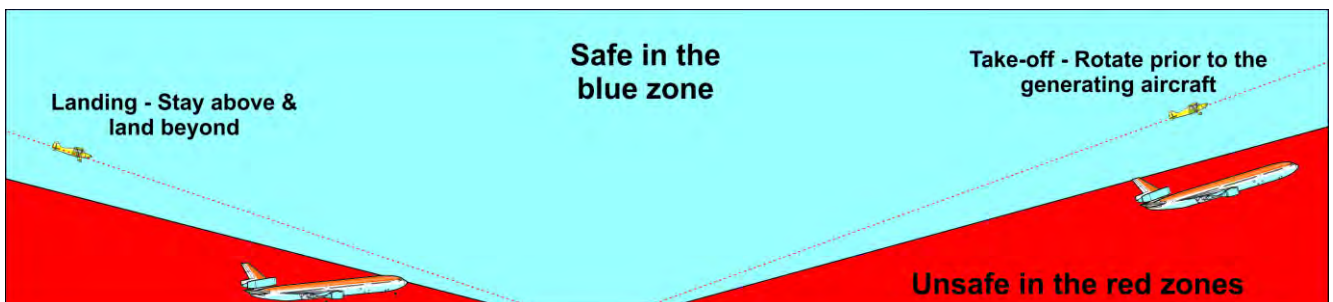
Fig. 86 Safe zones (blue) for landing and take-off in relation to wake turbulence generated by other aircraft.
